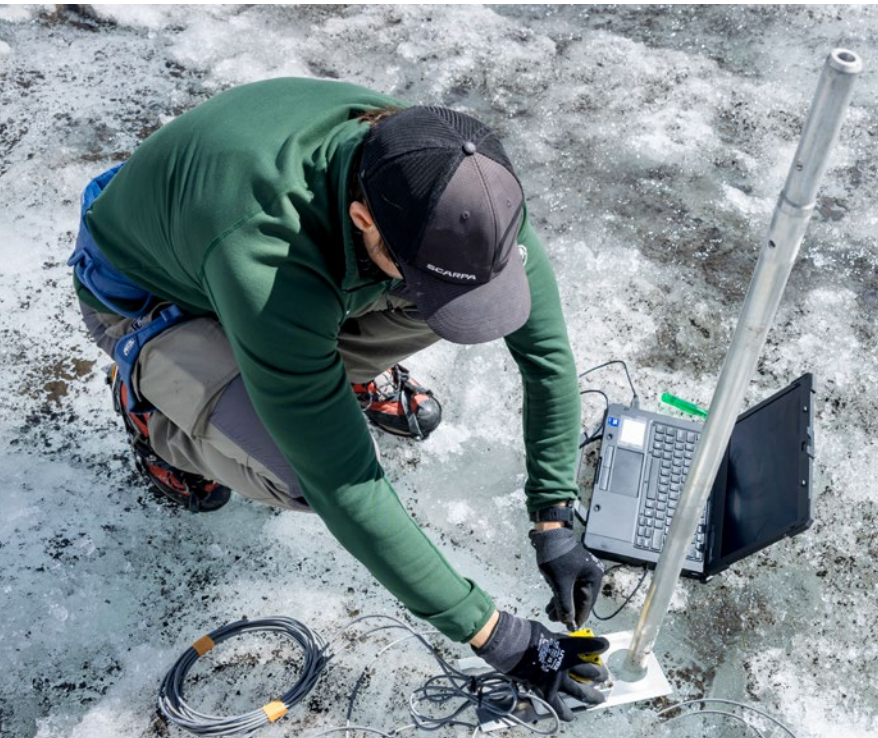
Glaciologist Janosch Beer downloads temperature data onto his laptop. The cable is connected to sensors that he inserted deep into the ice a few years ago.
