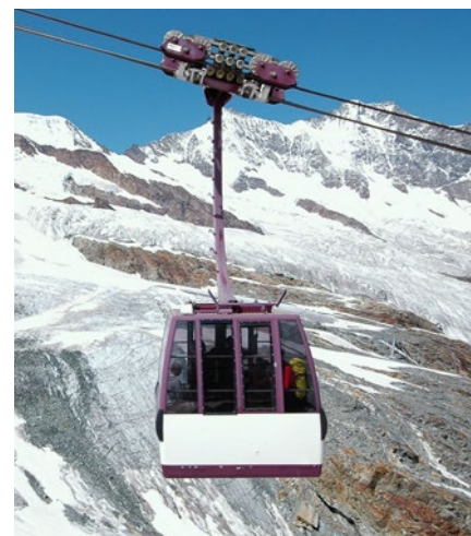
This system represents a remarkable piece of innovation. The world's first aerial cable car on three cables has been travelling up the mountain in Saas Fee since 1991. Photo: Martin Arnold
