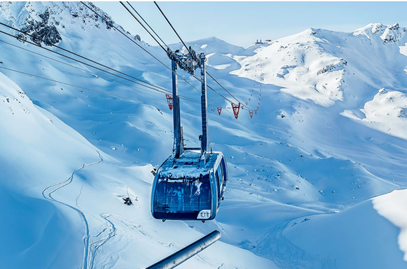
The "Urdenbahn" in Arosa and Lenzerheide is Switzerland's fastest cable car. The stanchion-free aerial tramway has connected two ski resorts since 2014 without having to open up new slopes. Photo: The Lenzerheide resort
